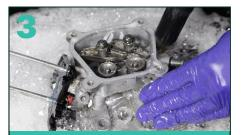
Heated to 42°C, the microbes become active in the ROwash Degreasing solution and eat the oil and grease turning them into harmless CO<sup>2</sup> and water – effectively recycling the fluid.
