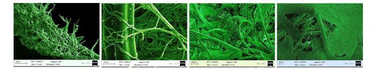
This bio film means that for the month-long life of the filter, there is a constant supply of microbes degrading the hydrocarbons and maintaining the optimum cleaning performance of the ROwasher.
